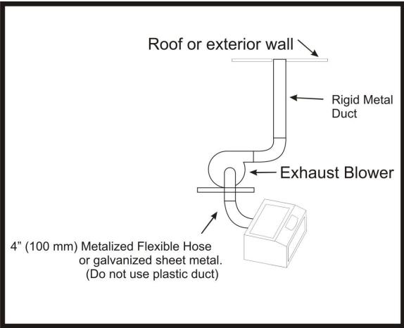
Example of typical exhaust setup.
