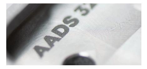
To change the surface color without penetrating the metal, the laser beam's focal point is crucial in achieving a dark mark. An annealed mark is accomplished with the focal point up (closer to) .070" to .110" (1.778 to 2.794 mm) or down (further away) -.060" to -.090" (-1.524 to -2.286 mm) from zero. Adjusting the speed, focus and frequency setting will vary the contrast of mark generally resulting in shades of blue, purple and black.
