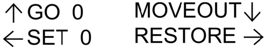
To set a new or temporary Table Home position, first move the table up or down using the joystick to focus on your material. Then, double center click to bring up the sub-menu. Tilt the joystick Up, Down, Left or Right to activate the associated menu item:
