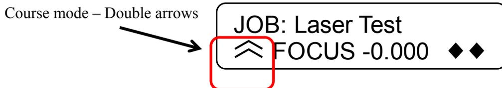
A single arrow indicates that you are in "Fine" adjustment mode and the table will move up or down in very small increments.
