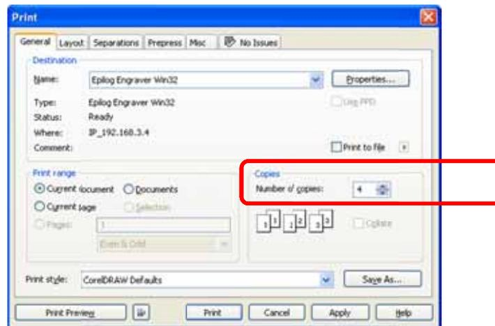
You can automatically engrave or cut a job multiple times by setting the Number of Copies to the number of passes that you want to make. When each pass is finished the laser will automatically start another pass until all passes are complete.
