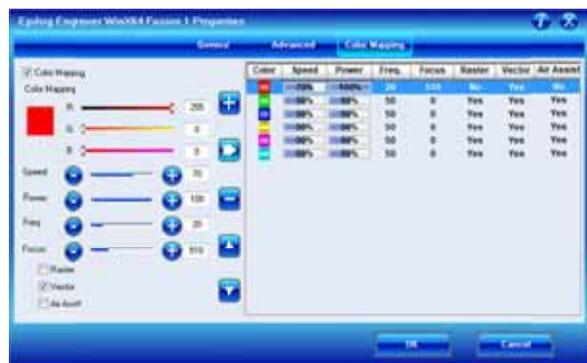
In our example we want to mark the green window frames first, so green must be the first color at the top of the list. Normally the color green is the second color down in the list. In order to move it we just select it and use the Up cursor to move it up one position.
